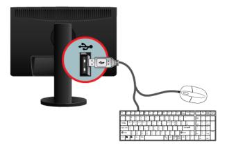
1. Connect the \*\* UP port of the monitor and the USB port of the computer with the USB cable.
